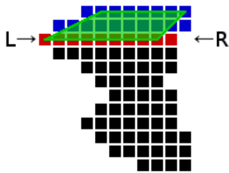
Figure 3d. In this case, the quad's edges are outside the next segment on both sides, so both the left and right limiting segments are set to the new segment.
